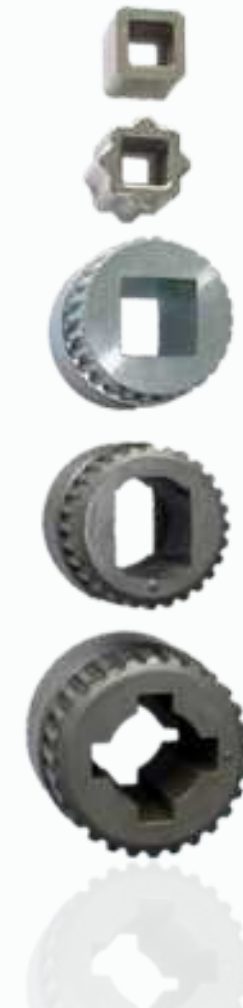
Drive bush is used for mechanical connection between a quarter-turn actuator and a valve shaft. There are various machinings available such as square, double d, keyway.
